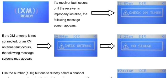
number, or press the select button twice; a beep occurs and the scroll wheel can be used to browse the channel list
